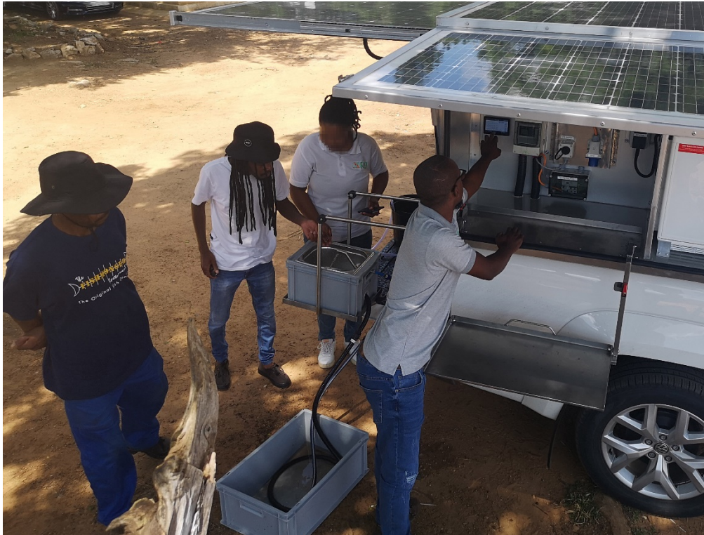
The prototype of a care unit provides storage space and the energy supply for diverse medical devices, active substances and tests. © Fraunhofer ISE
